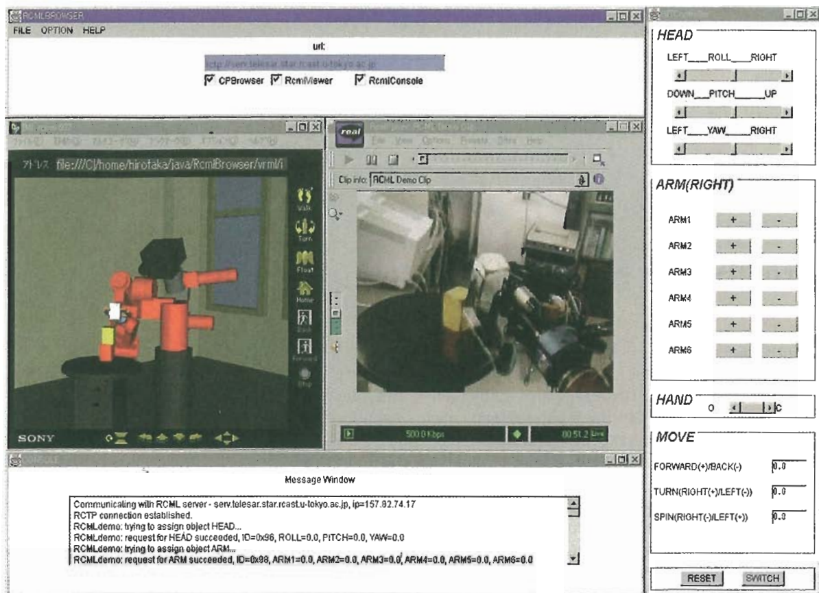
6 An example of an RCML browser displaying the VRML image of the robot (left), the TV image (right), and the optional text communicator (bottom).
