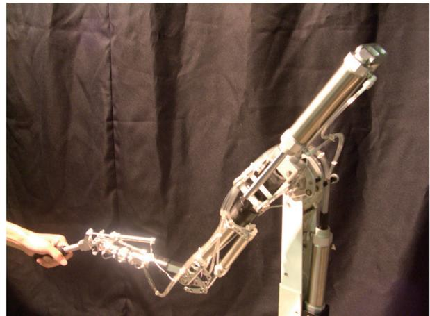
Fig. 1 Robot arm using pneumatic cylinder.
