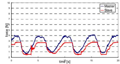
**Fig. 14** Force on the arm in impedance control type
