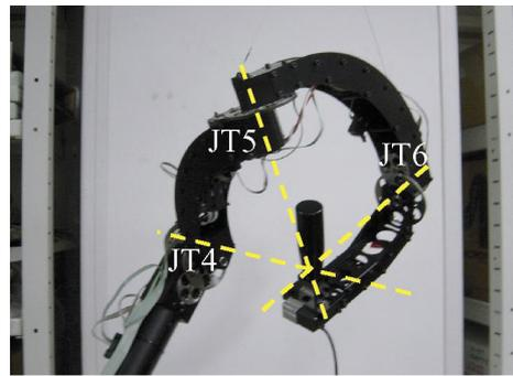
**Fig. 3** The three axes of the wrist cross at one point
