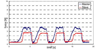
**Fig. 12** Force on the arm in symmetry type
