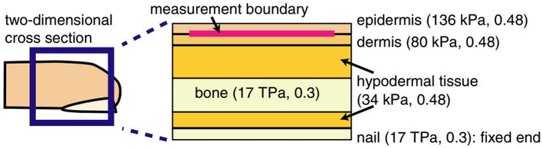
**Fig. 2.** Constructed fingertip model. We set the nail as the fixed end. Young’s modulus and Poisson’s ratio are indicated in the parentheses.
