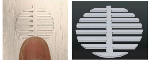
Figure 1: An example of the pattern for inducing an illusionary concave shape. The shape shown on the left is a milled aluminum plate, and the right is a CAD model of this pattern.
