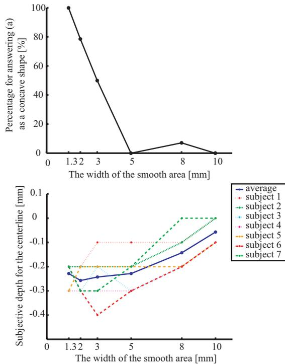
Figure 4: Results of experiment 1. Top: Fraction of subjects choosing the illusory concave shape in preference to the actual concave shape. Bottom: Subjective depth of the test plate selected by comparison with the reference stimulus plate in Figure 3.
