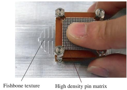
Figure 8: Rubbing fishbone tactile pattern with a high density pin matrix. Stroking the test pattern with a pin matrix, which delivers only vertical height information to fingertip.
