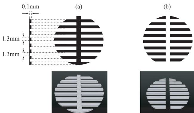
Figure 2: Machined aluminum stimulus plates containing two complementary stimuli and corresponding CAD models. (a) Illusory concave shape (actual convex shape) (b) Concave shape, reversing the height distribution of (a). Black areas are raised 0.1 mm above white areas.
