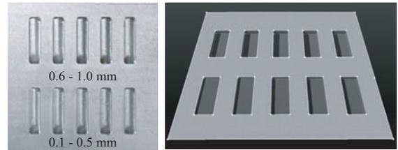
Figure 3: Reference stimulus metal plate and CAD model. The depth increased by 0.1 mm in successive grooves. Width of the grooves is 5 mm. Subjects compared this reference stimulus and test stimulus sets to evaluate the subjective depth perception.
