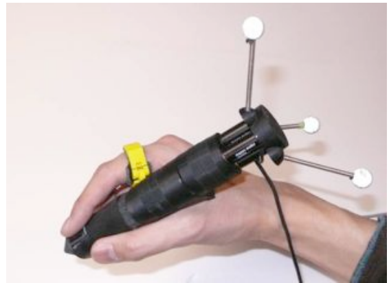
Figure 1. Ungrounded pen-shaped kinesthetic display
