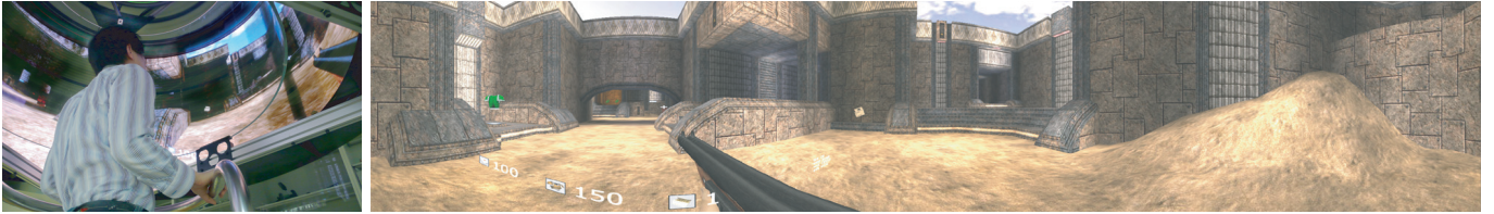
Figure 1: Left: The appearance of TWISTER IV (Telexistence Wide-angle Immersive STEReoscope model IV). Right: We selected the open source first person shooting game Cube ( http://cubeengine.com/ ) and rendered it by using our method. This figure shows immersive stereoscopic images for left eye ( 1584 \times 600 [pixel]). The method could render stereo images of Cube at 20–30fps.
