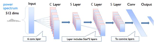
**Figure 4:** Machine learning for dual-layered tactile recognition: convolution layer and a subsampling layer for the neural network [Krizhevsky et al. 2012].
