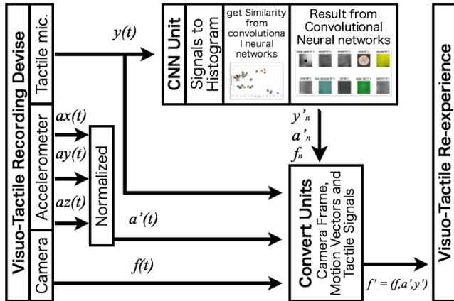
**Figure 6:** Proposed architecture for displaying recorded data and recognizing vibro-tactile waves. In this case, we used a convolutional neural network.
