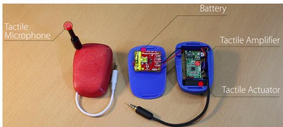
**Figure 3:** Attachment overview: microphone includes an embodied probe; captured signals convey audio through a jack attached to the smartphone; the vibro-tactile wave is displayed using a tactile actuator through a tactile amplifier from the smartphone.
