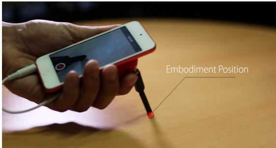
(a) Recording contacted textures using an embodied probe
