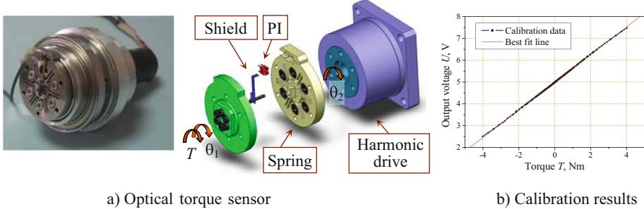
a) Optical torque sensor
