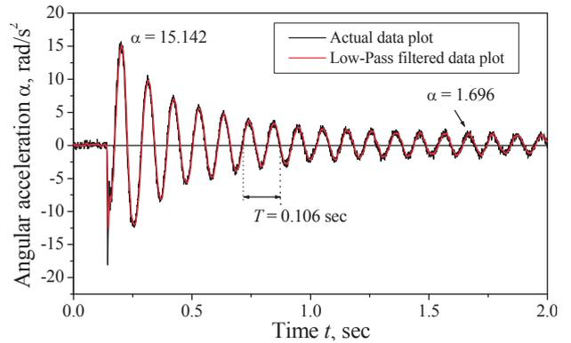
Fig. 8 Impulse response of the robot link.
