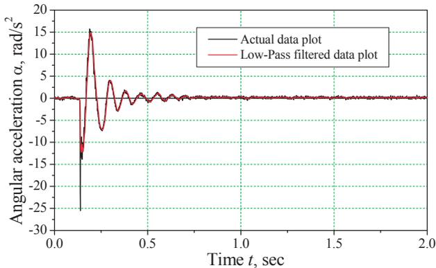
Fig. 12 Impulse response of system with controller.
