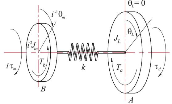
Fig. 5 Two-inertia vibration model of robot joint.
