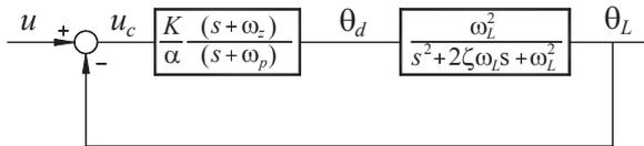
Fig. 9 System with lead compensator.
