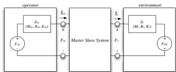
Fig. 6 Impedance representation of the operator, master-slave system and environment
