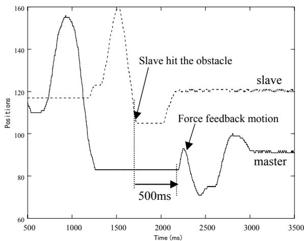
Fig.9 The slave hit the obstacle with 500ms time delay
